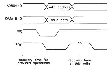
Figure 4. Timing Diagram of Processor Interface When Writing
