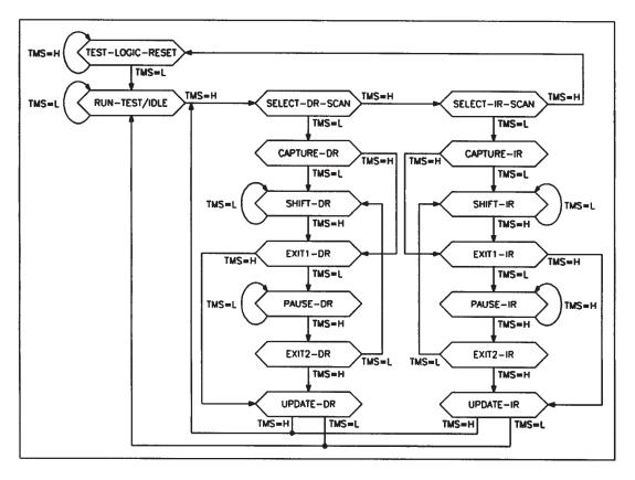
Figure 21. IEEE Std 1149.1 Test Access Port (TAP) Status Diagram
