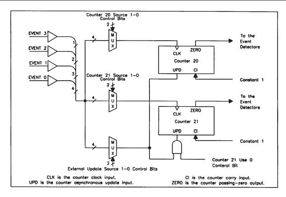
Figure 15. COUNTER20 and COUNTER21 Configured as Separate 16-Bit Counters
