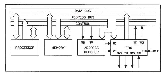
Figure 3. Connection of the TBC to a Microprocessor
