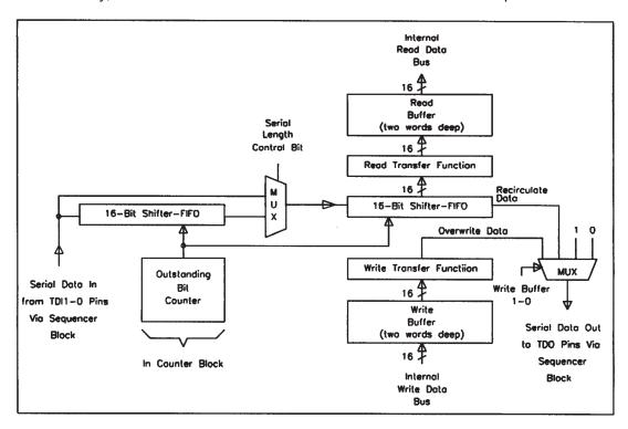
Figure 12. Serial Block
