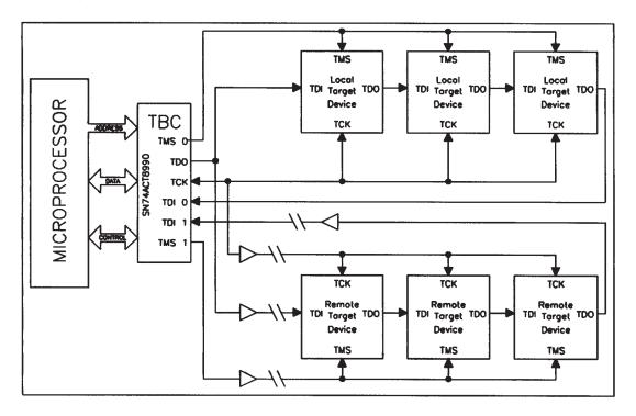
Figure 8. Connection of Several IEEE Std 1149.1 Test Buses to the TBC, With Buffering of the Test Bus Signal
