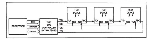
Figure 1. Test System With TBC SN74ACT8990
