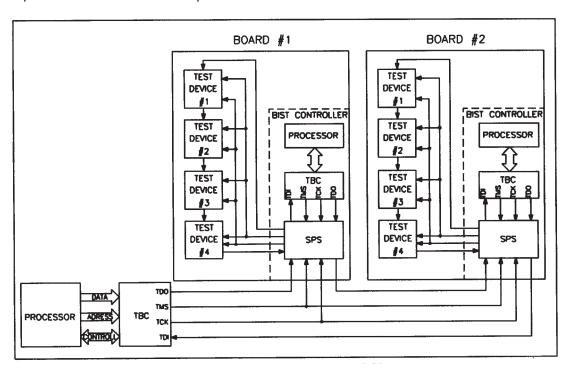
Figure 2. System With Built-In Self-Test (BIST)
