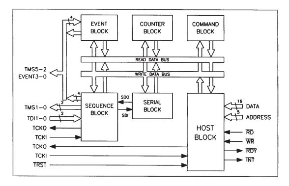
Figure 9. Block Diagram of TBC SN74ACT8990
