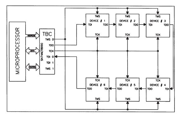
Figure 6. Connection of a IEEE Std 1149.1 Test Bus to the TBC
