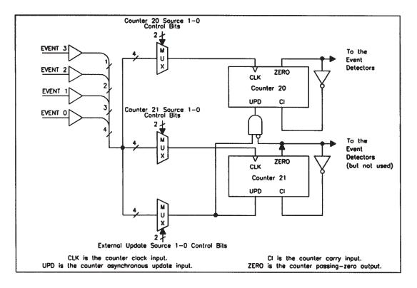
Figure 16. COUNTER20 and COUNTER21 Configured as Combined 16-Bit Counters
