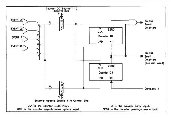
Figure 17. COUNTER20 and COUNTER21 Configured as One 32-Bit Counter (COUNTER2)
