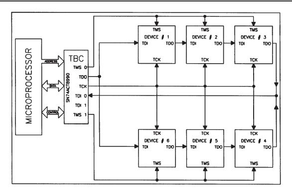
Figure 7. Connection of Two IEEE Std 1149.1 Test Buses to the TBC
