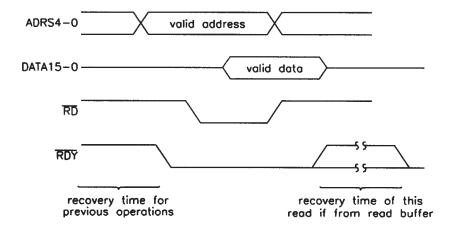
Figure 5. Timing Diagram of Processor Interface When Reading
