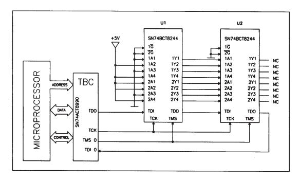
Figure 22. Hardware Example: Two SCOPE Octals SN74BCT8244N
