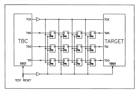
Figure 11. Link-Delay Logic
