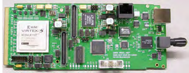
Figure 4. Prototype UW SLHC Calorimeter Trigger Card (Aux Card).
