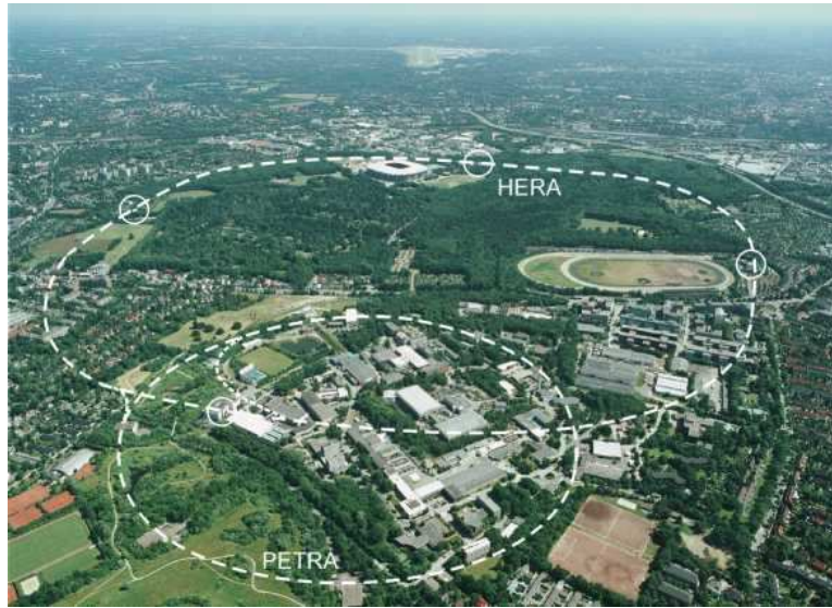
Figure 3.1: An aerial view of DESY. The white dashed lines show the underground locations of PETRA and HERA and the small white circles show the location of the detectors.
