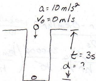
$$d = \frac{1}{2} a t^2 = \frac{1}{2} (10 \text{ m/s}^2) (3 \text{ s})^2 = 5 \frac{\text{m}}{\text{s}^2} \times 9 \text{ s}^2$$
