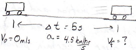
$$a = \frac{\Delta V}{\Delta t} = \frac{V_f - V_0}{\Delta t}$$
