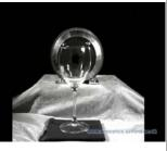
Stroboscopic movie of fundamental vibration mode of a wineglass
