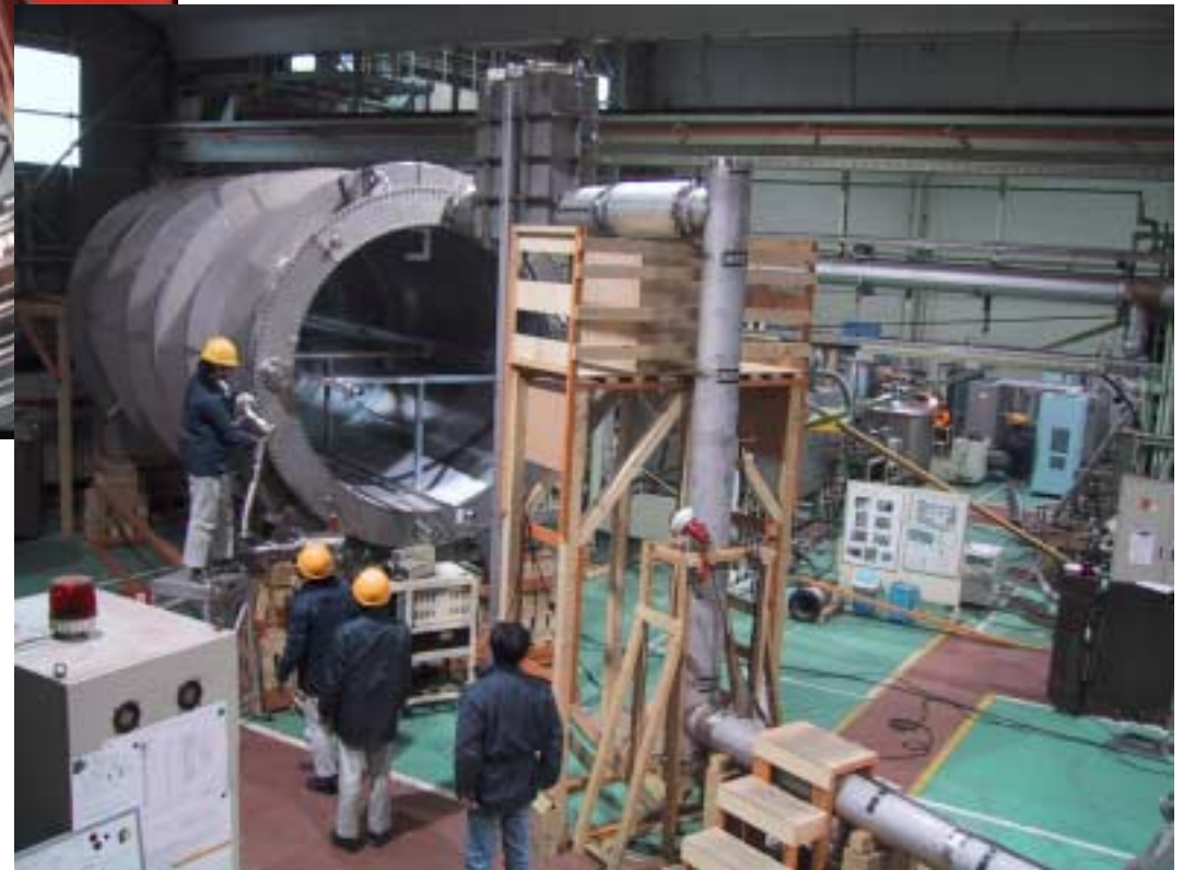
Completed ATLAS solenoid and cryogenics chimney during tests at Toshiba (for KEK)
