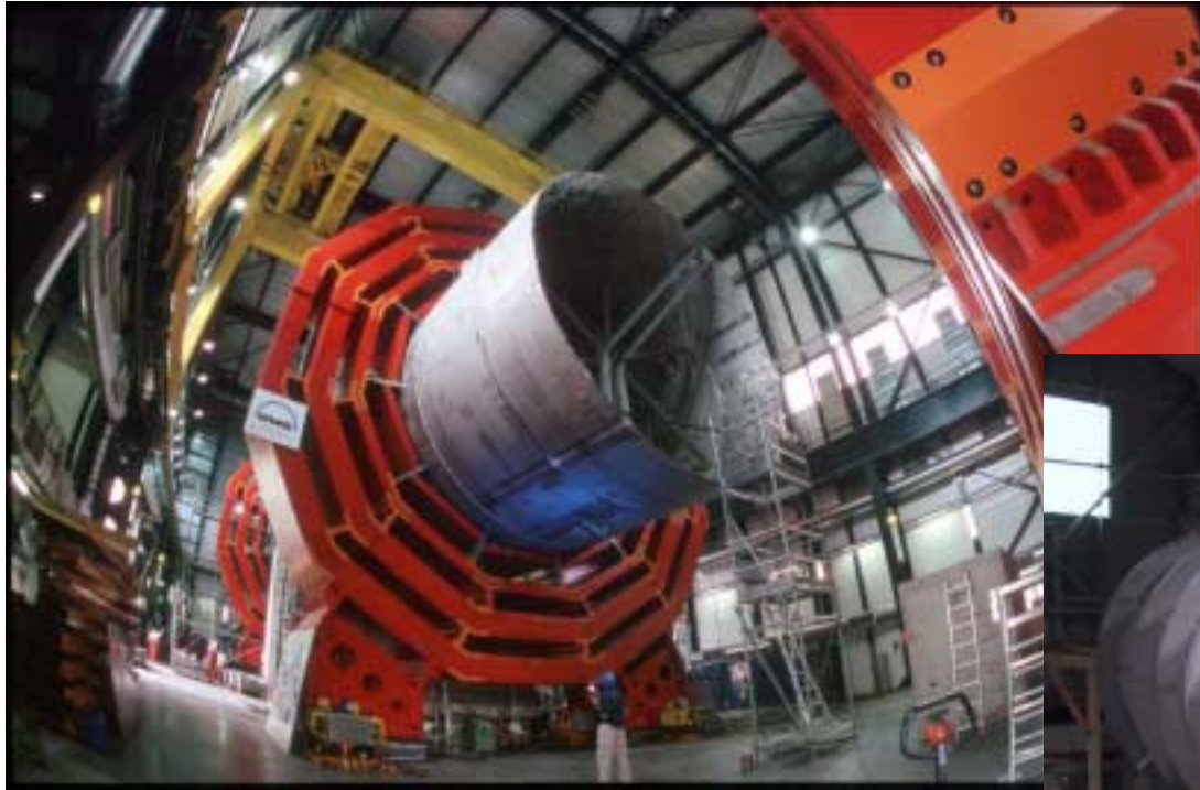
CMS barrel yoke wheels assembled at SX5 (point 5) Central wheel supports the coil, barrel HCAL, ECAL and tracker
