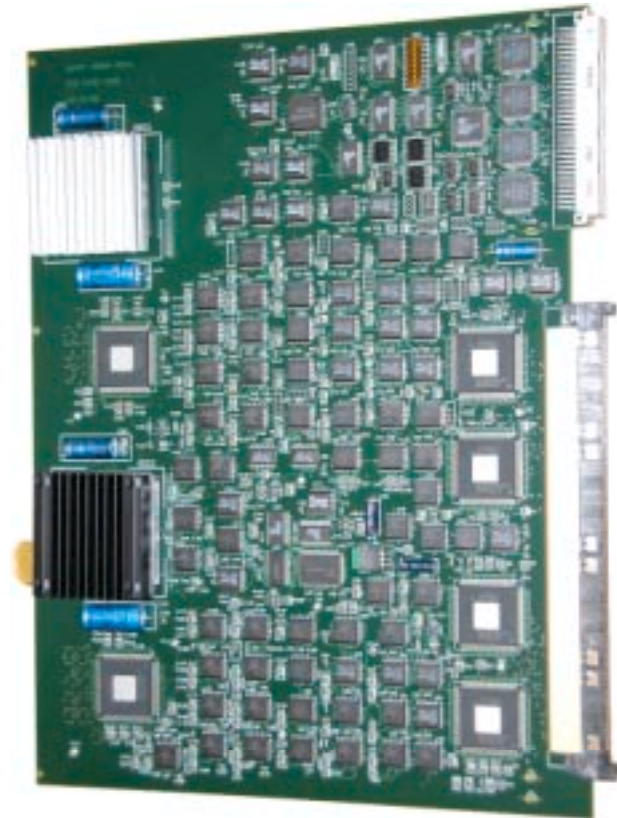
Figure 7. Pre-production Electron Isolation Card with Electron ID and Sort ASICs installed.
