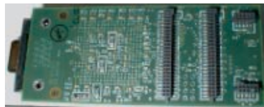
Figure 5. Pre-production 4 Gbit/s Copper Receiver Mezzanine Card.
