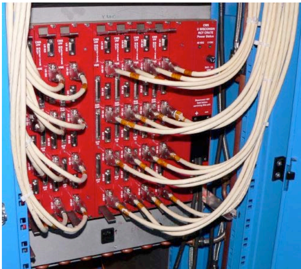
Rear of Full RCT crate fully cabled to HCAL trigger primitive logic
