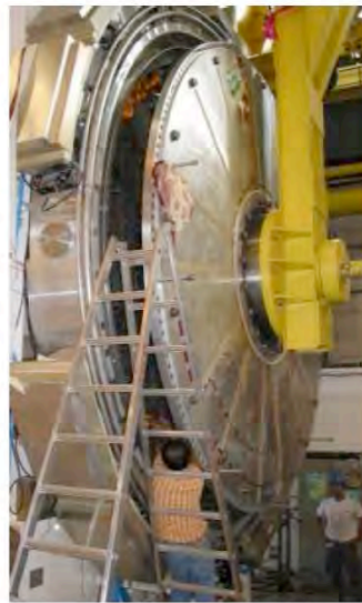
REMOVE COLD COVER TO EXPOSE REAR FACE OF HEC2
