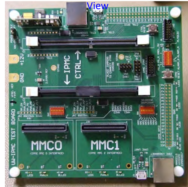
ZYNQ-IPMC Test Fixture Top View
