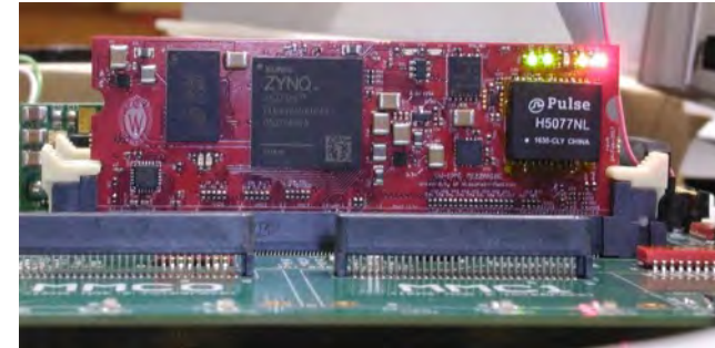
ZYNQ-IPMC in Test Fixture
