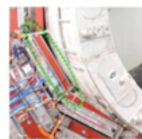
Outer (HO) scintillator tiles outside yoke 1 or 2 longitudinal layers 10mm scint coverage: |\eta| < 1.3
