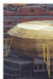
Endcap (HE) Two brass endcap discs 19 longitudinal layers 8cm brass + 3.7mm scint coverage: 1.3 < |\eta| < 3.0
