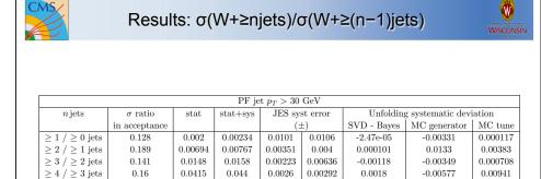
Table 8.4: Results for cross section ratio  $\sigma(W + \ge n \text{ jets})/\sigma(W + \ge (n-1) \text{ jets})$  within the acceptance with inclusive jet counting. Sources of uncertainty shown are statistical, statistical + uncorrelated systematics (fit and efficiency), correlated systematics (jet energy scale, JES), and deviations when using different unfolding methods (algorithm, generator, and tune).
