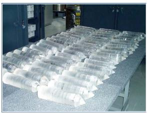
Although the pixels used in PET scanners are small (typically  $3x3x20mm^3$ ), they are cut from large ingots, about 5cm in diameter and 20 to 25 cm in length, grown by Czokralski technology.
