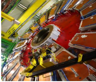
Figure 24: De Bryun and Sreekala prepare to extract a CSC chamber
